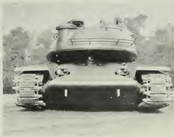
HYDRO-PNEUMATIC suspension system for tanks, developed by Army, will enable them to change ground clearance.
